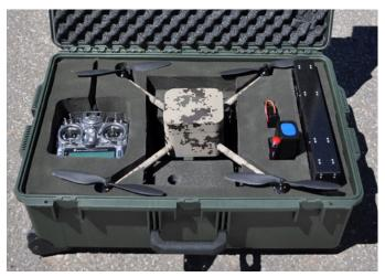
Leptron used Stratasys FDM technology to make complex fuselage parts on its five-pound remotely piloted RDASS (rapidly deployed aerial surveillance system).
