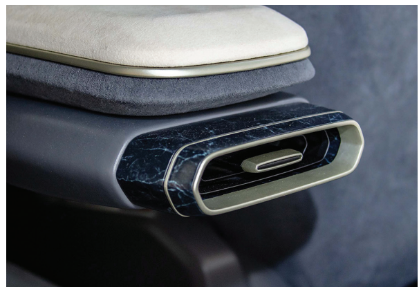
3D printed air conditioning diffuser with marble effect, made with the Stratasys J750.
